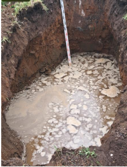
Photo 6 – Trial Hole T1 Water Fill: Level of effective depth at proposed invert (75% level of fill). Water level = 0.9m deep
