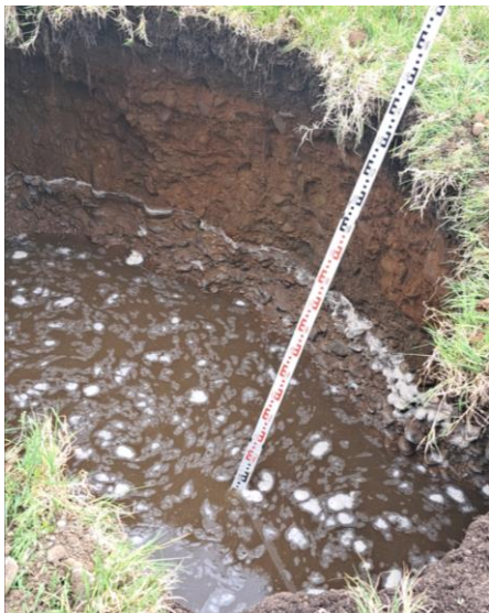
Photo 11 – Trial Hole T2; Water Fill: Level of effective depth at proposed invert (75% level of fill). Water level = 0.825m deep. (dimensions 1.2m wide x 1.6m long)
