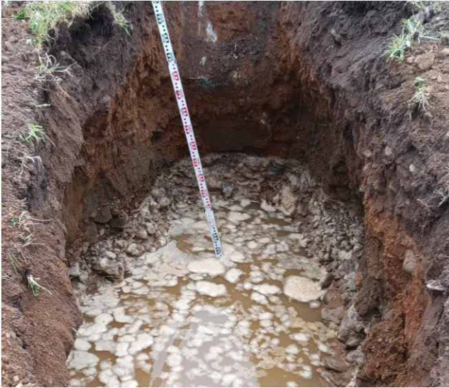
Photo 17 – Trial Hole T3; Water Fill: Level of effective depth at proposed invert (50% level of fill). Water level = 0.75m deep. (dimensions 1.0m wide x 2.0m long)
