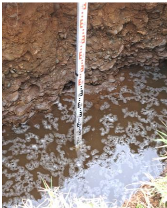
Photo 21 – Trial Hole T4; Water Fill: Level of effective depth at proposed invert (50% level of fill). Water level = 0.550m deep. (dimensions 1.0m wide x 2.0m long)
