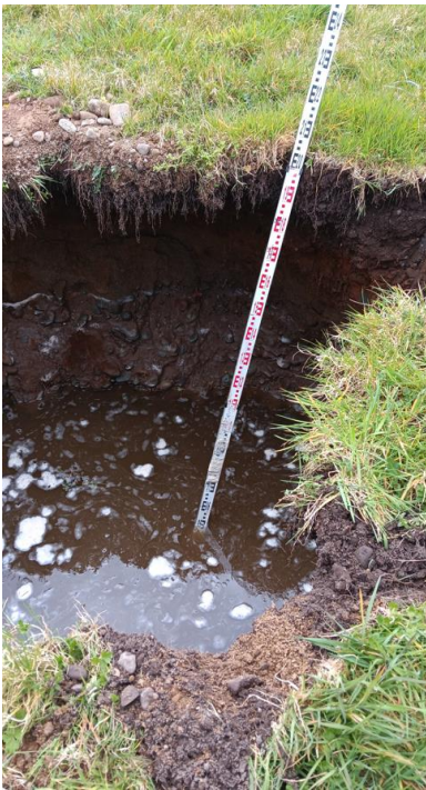
Photo 25 – Trial Hole T5; Water Fill: Level of effective depth at proposed invert (50% level of fill). Water level = 0.55m deep. (dimensions 1.5m wide x 1.8m long)
