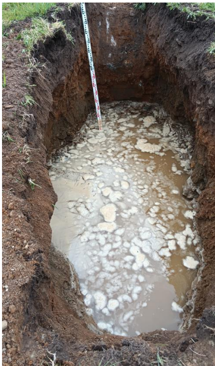
Photo 15 – Trial Hole T3; Water Fill: Level of effective depth at proposed invert (100% level of fill). Water level = 1.4m deep.
