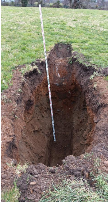
Photo 14 – Trial Hole T3 depth = 2.65m (see Trial hole Data log) (hole dimensions: width = 1.0m, length = 2.0m.)
