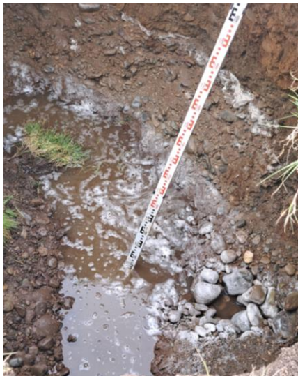
Photo 13 – Trial Hole T2; Water Fill: Level of effective depth at proposed invert (25% level of fill). Water level = 0.275m deep. (dimensions 1.2m wide x 1.6m long)
