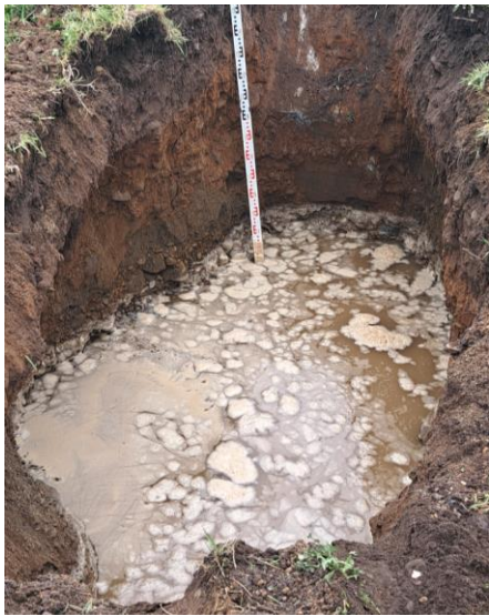
Photo 7 – Trial Hole T1 Water Fill: Level of effective depth at proposed invert (50% level of fill). Water level = 0.6m deep
