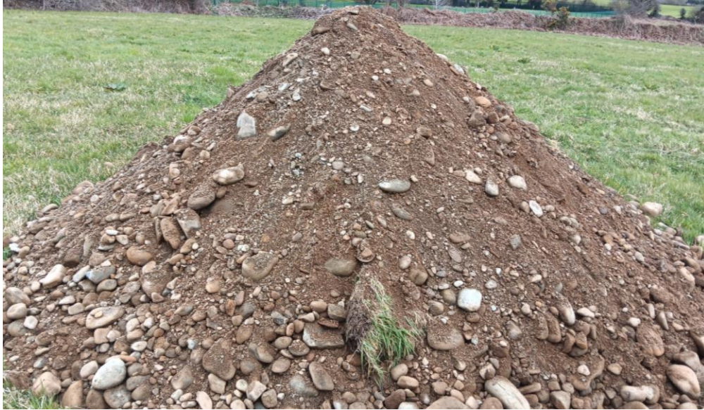
Photo 28 – Trial Hole T3; Spoil from excavation: heterogenous soil: sandy gravel with minor silt content. Some sporadic cobbles (<200mm). No boulders present.
