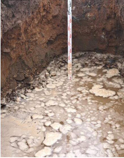
Photo 8 – Trial Hole T1 Water Fill: Level of effective depth at proposed invert (25% level of fill). Water level = 0.3m deep
