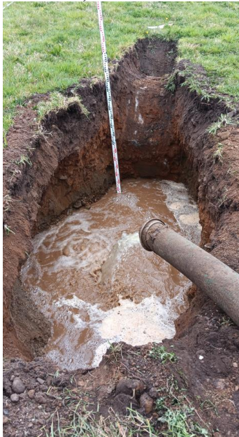
Photo 14 – Trial Hole T3 depth = 2.65m (see Trial hole Data log) (hole dimensions: width = 1.0m, length = 2.0m.)
