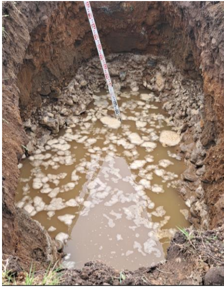
Photo 20 – Trial Hole T4; Water Fill: Level of effective depth at proposed invert (75% level of fill). Water level = 0.675m deep. (dimensions 1.0m wide x 2.0m long)
