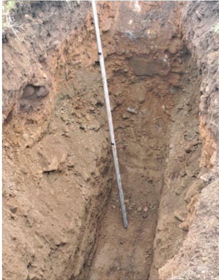
Photo 4 Soil Strata – Trial Hole T1, depth = 2.65m (see Trial hole Data log) (hole dimensions: width = 1.0m, length = 2.0m.)
