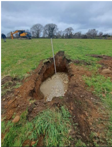
Photo 5 – Trial Hole T1 Water Fill: Level of effective depth at proposed invert (100% level of fill). Water level = 1.2m deep.
