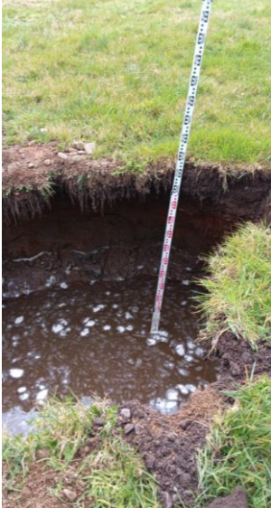
Photo 24 – Trial Hole T5; Water Fill: Level of effective depth at proposed invert (75% level of fill). Water level = 0.825m deep. (dimensions 1.5m wide x 1.8m long)
