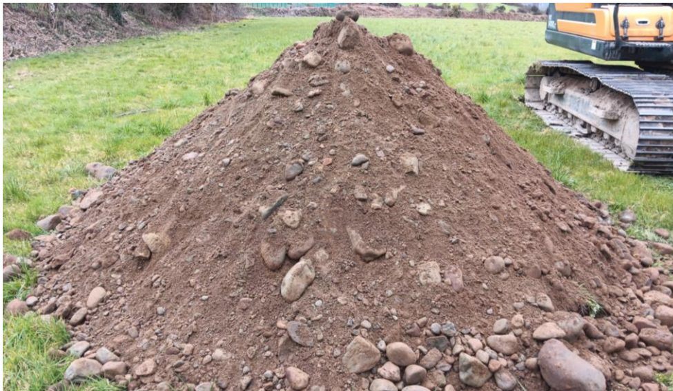
Photo 29 – Trial Hole T5; Spoil from excavation: heterogenous soil: sandy gravel with minor silt content. Some sporadic cobbles (<200mm). No boulders present.
