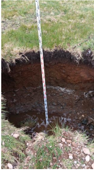
Photo 26 – Trial Hole T5; Water Fill: Level of effective depth at proposed invert (25% level of fill). Water level = 0.275m deep. (dimensions 1.5m wide x 1.8m long)
