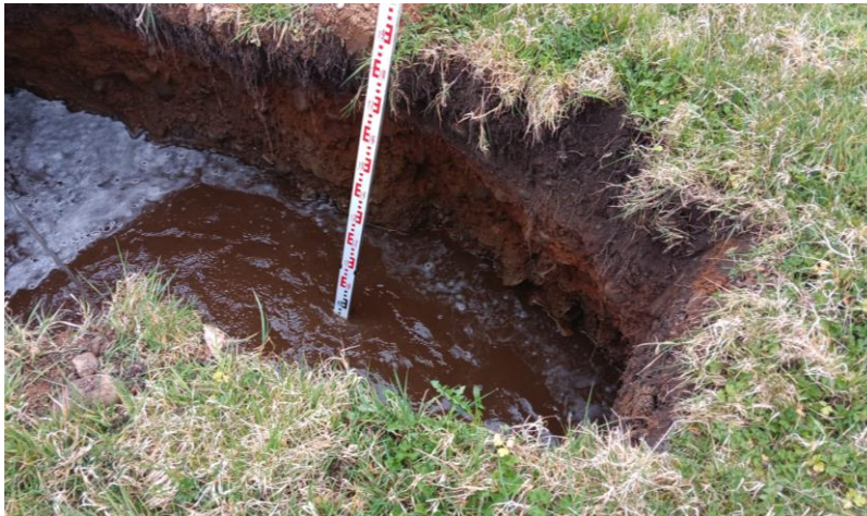
Photo 19 – Trial Hole T4; Water Fill: Level of effective depth at proposed invert (100% level of fill). (1.9m deep) Water level = 0.9m deep. (dimensions 1.0m wide x 2.0m long)
