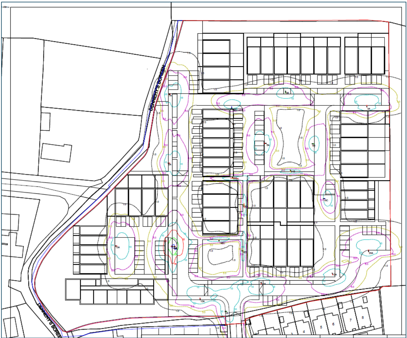
Illustration 4.1. Extract (clip) from 1:500 A1 Public lighting drawing Illumination contours.
