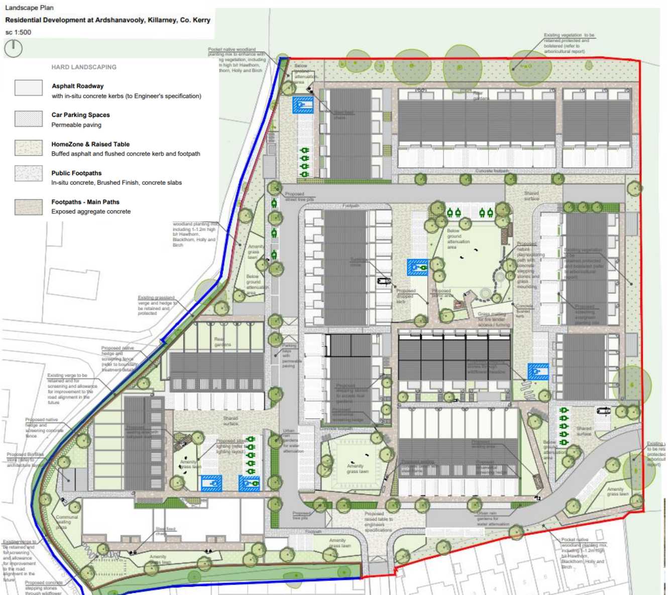
Figure 5 Layout showing the surface changes within the development to signify pedestrian priority Areas
